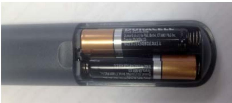
**Figure 3: Batteries should go in like this**
